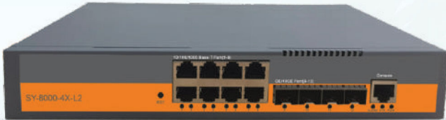
SY-8000P-4X-L2 8*10/100/1000Mbps Base-T 4*1000M Base-X SFP/10GE SFP+
