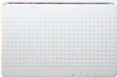
SY-1005 5*10/100/1000M auto-negotiation RJ45 ports (Auto MDI/MDIX) RJ45 ports (Auto MDI/MDIX)
